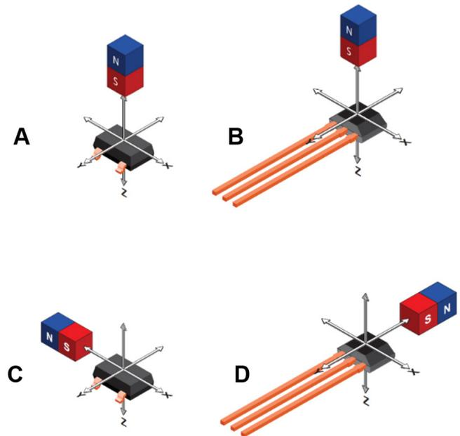
Figure 6: Magnetic Sensing Orientations
