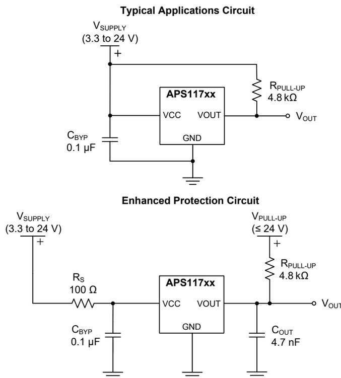
**Figure 7: Typical and Enhanced Protection Application Circuits**
