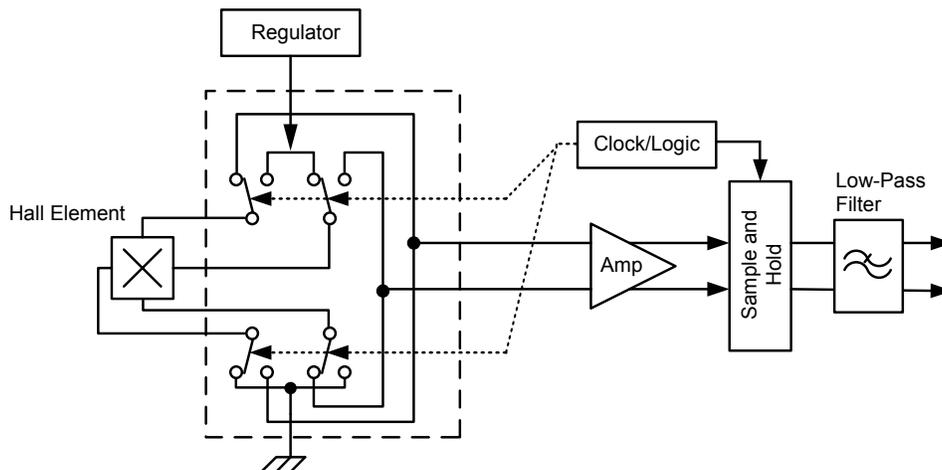
**Figure 8: Model of Chopper Stabilization Circuit
