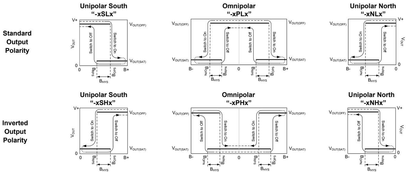
**Figure 3: Hall Switch Output State vs. Magnetic Field**
