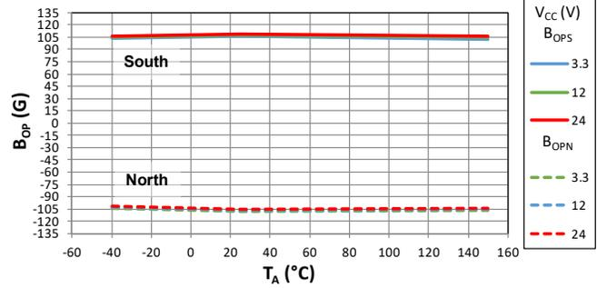
Average Release Point versus Supply Voltage
