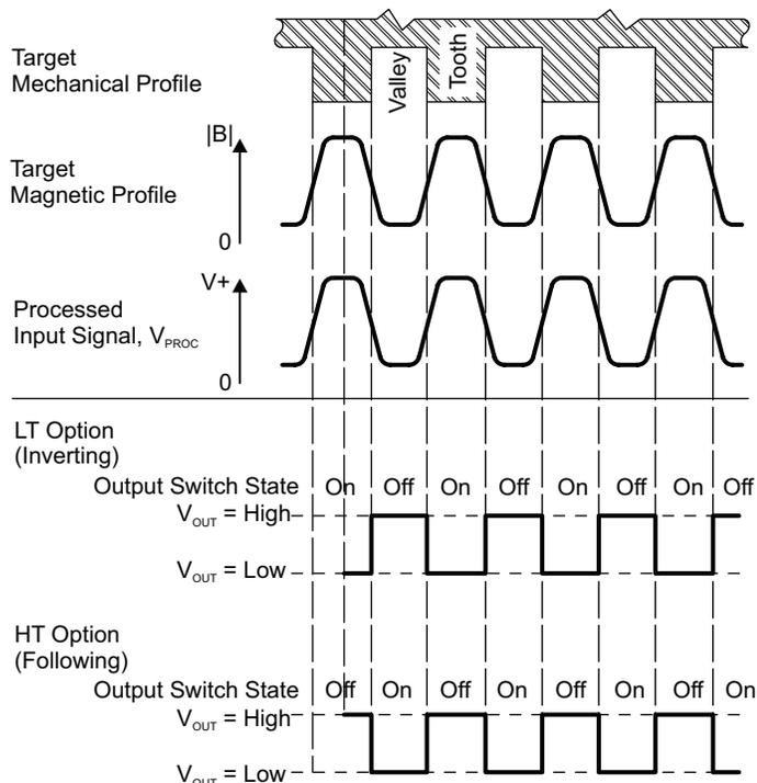
**Figure 4: Output Polarity**
