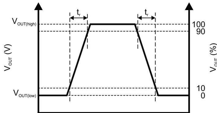
**Figure 2: Output Rise Time and Output Fall Time**
