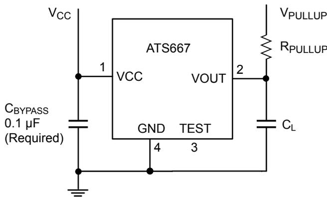
Figure 6. Typical circuit for proper device operation.
