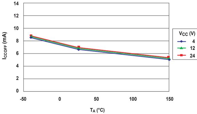
Supply Current (Off) versus Supply Voltage
