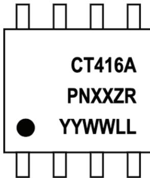
Figure 21: CT416 Device Marking for 8-lead Package
