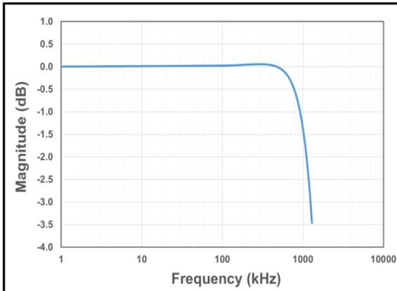
Figure 7: CT416 Bandwidth with  $C_{FILTER} = 1.0\ \text{pF}$
