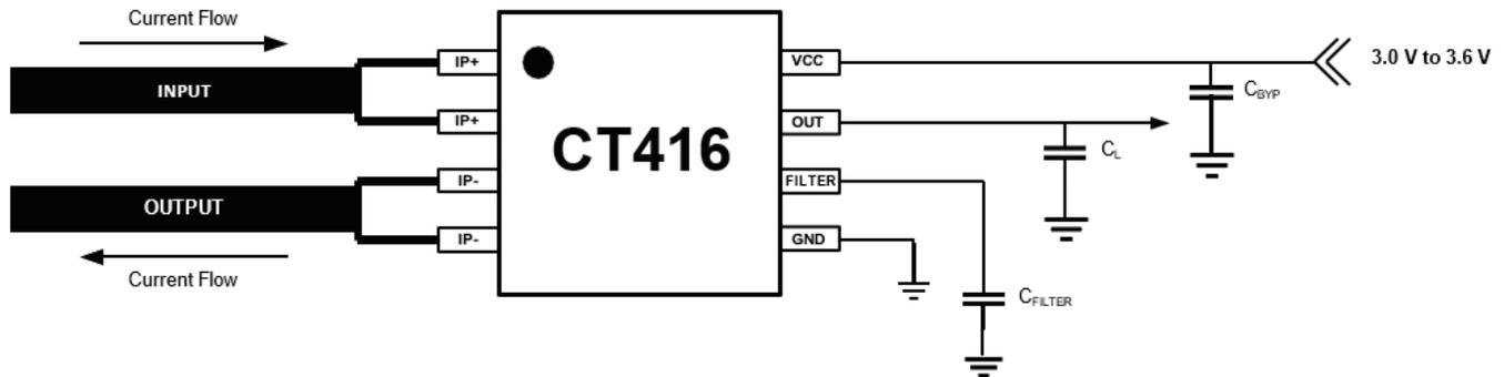
Figure 2: CT416 Application Block Diagram
