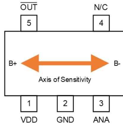
**Figure 4: CT8152 5-Lead SOT23 Package for Analog Output**
