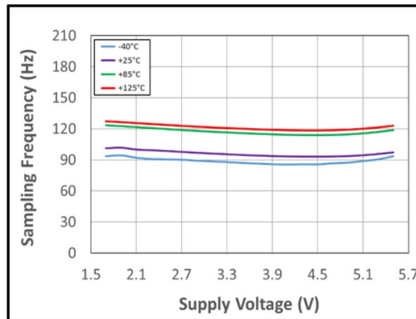
Figure 26: Sampling Frequency vs. Supply Voltage vs. Temperature
