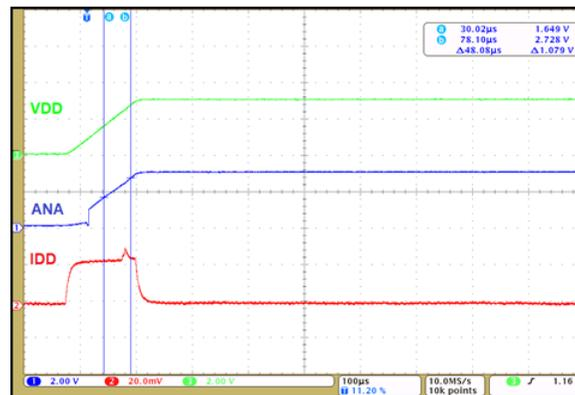
Figure 7: Power-On Time for Analog Output
