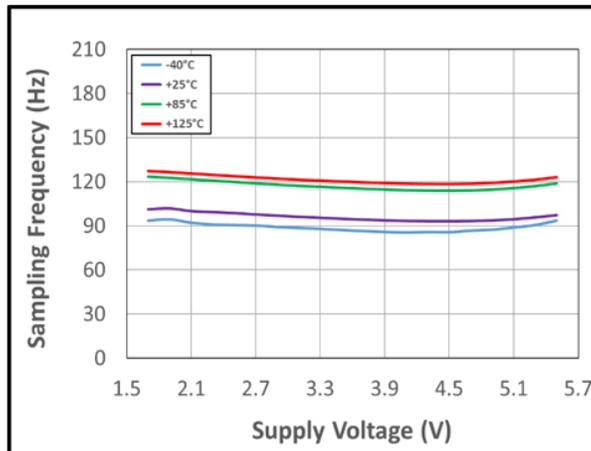
Figure 13: Sampling Frequency vs. Supply Voltage vs. Temperature
