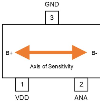
**Figure 3: CT8150 3-Lead SOT23 Package for Analog Output**
