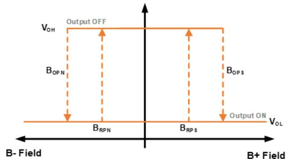
Figure 29: CT8152 Output Behavior vs. Magnetic Field
