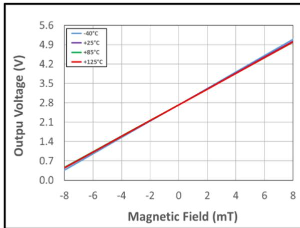
Figure 10: Output Voltage vs. Magnetic Field over Temperature at  $V_{DD} = 5.5\text{ V}$
