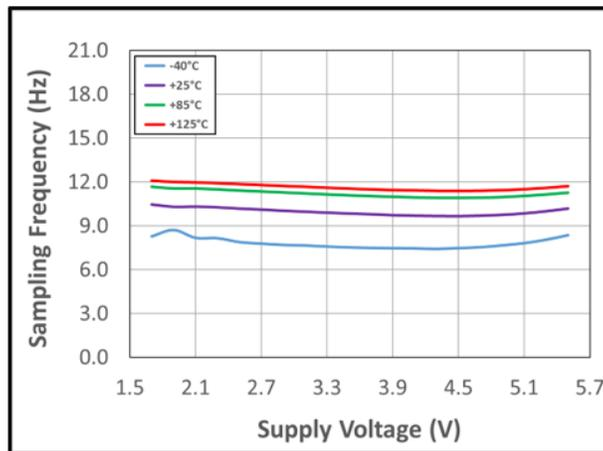
Figure 23: Sampling Frequency vs. Supply Voltage vs. Temperature
