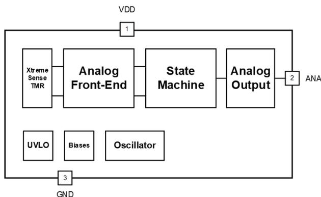
**Figure 1: CT8150 with Analog Output Block Diagram**
