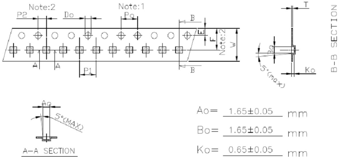
Figure 43: Tape and Pocket Drawing for LGA-4 Package
