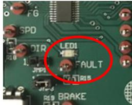
**B.** The problem is likely lock detection. If so, go to the Standby / Protection page and disable all the lock detect features.
