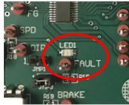
**B.** If the LED is off, connect a current probe and voltage probe to the motor outputs and check if there is any current / voltage output to the motor phase. If there is voltage but no current, check motor phase connections.
