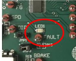
**B.** If it is OCP, check the phase output wire connections.
