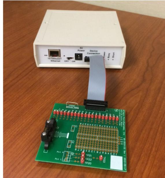
**Figure 2: Ribbon Cable Attached to the Daughter Board and the ASEK05**
