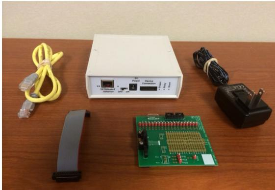
**Figure 1: Components of the ASEK05**
