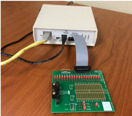
**Figure 3: Ethernet Cable and Power Supply Attached to the ASEK05**
