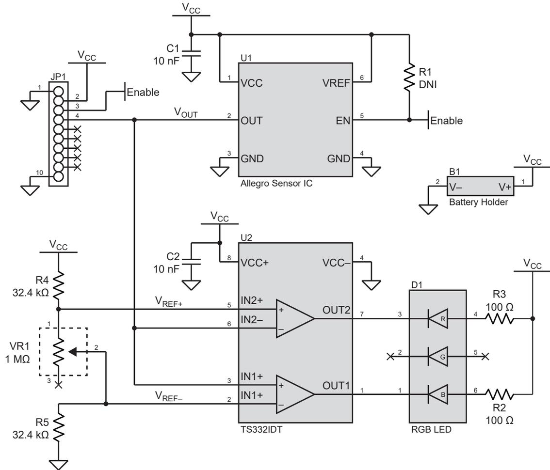
Figure 2: Analog 1D Linear Demo Schematic
