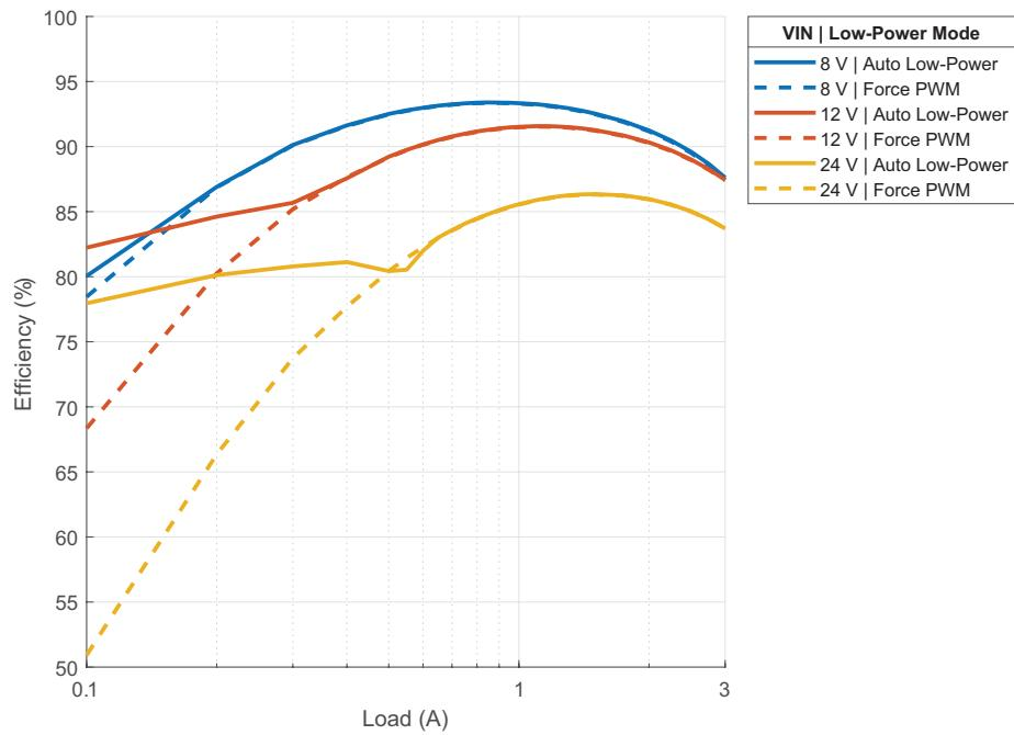
Figure 6: Efficiency at  $V_{OUT} = 5$  V,  $f_{SW} = 2.15$  MHz
