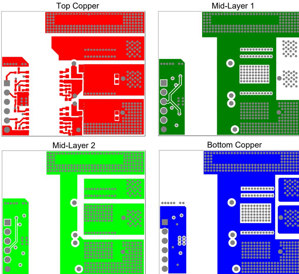
Figure 13: APEK85111KNH-01-T-MH PCB Copper Layers
