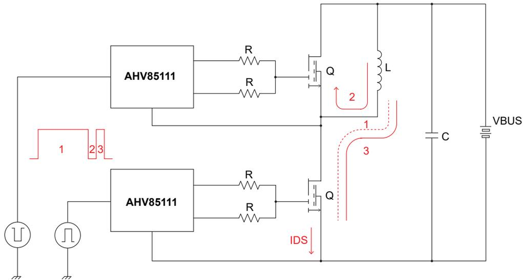
**Figure 7: Double-Pulse Test**
