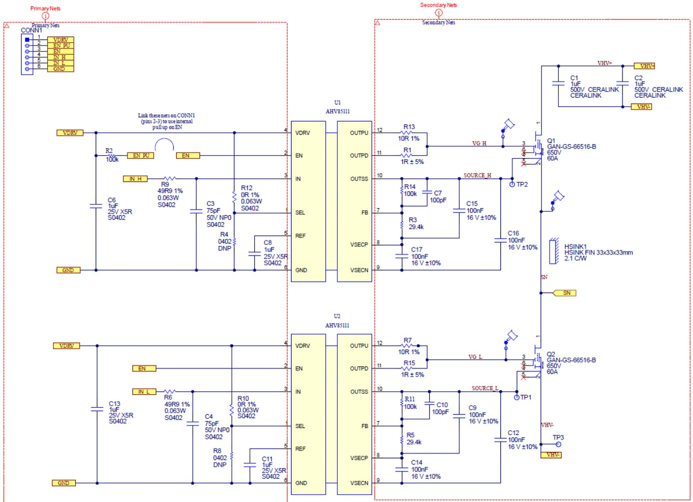
Figure 11: APEK85111KNH-01-T-MH Schematic
