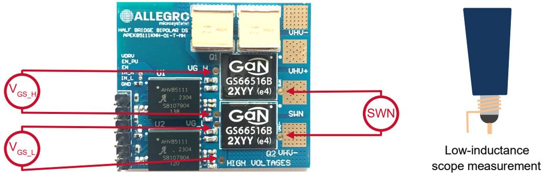
Figure 5: Measurements Points
