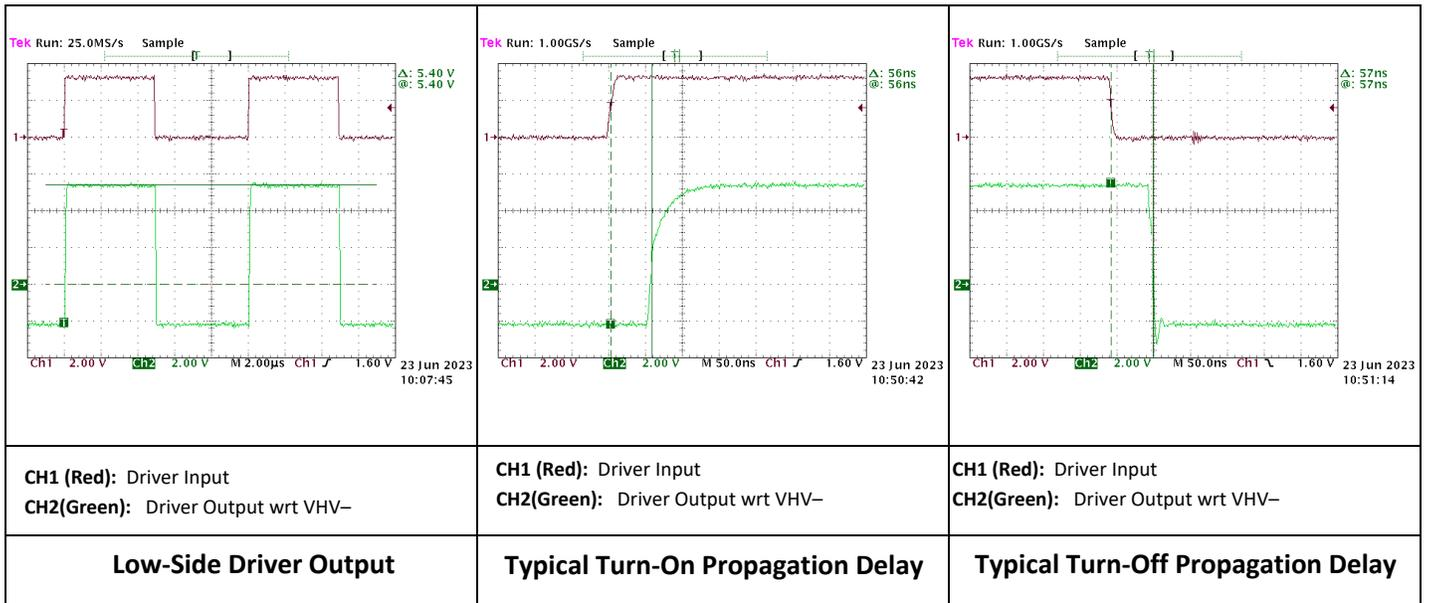
Figure 6: Typical Driver Output at 100 kHz
