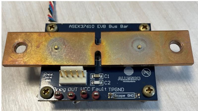
**Figure 3: ASEK37610 Test Point Connections**
