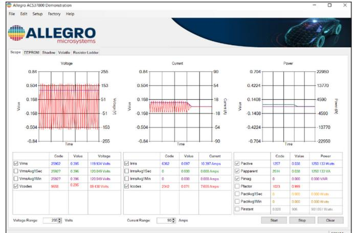
Figure 19: Example Scope Mode
