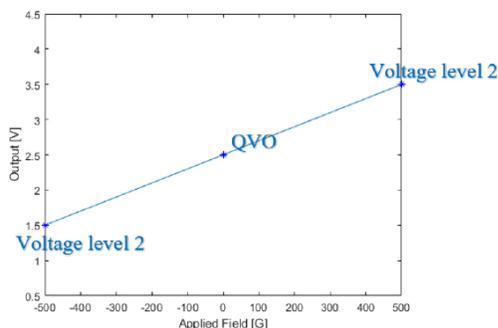
Figure 26: Calculating sensitivity using two known points
