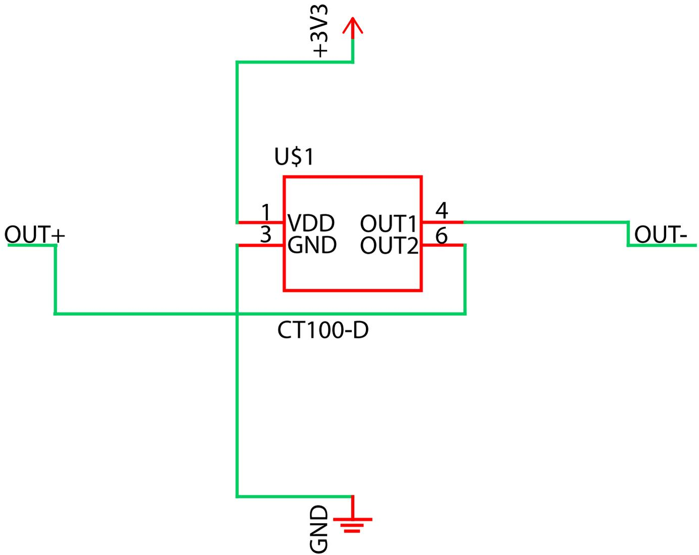
Figure 3: EVB102 SOT23-6 evaluation board schematic
