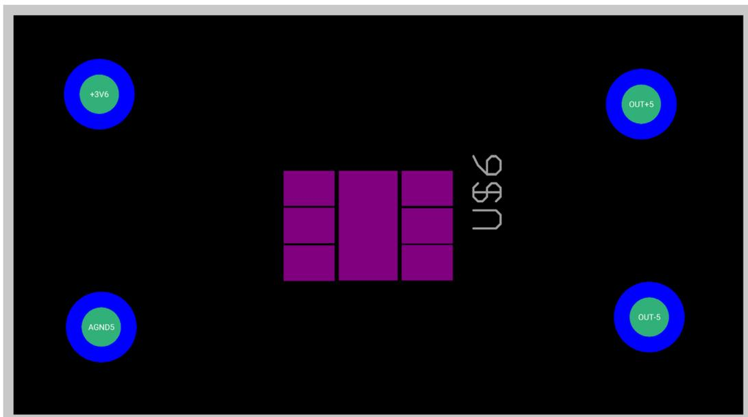
Figure 5: EVB102 SOT23-6 evaluation board bottom layer
