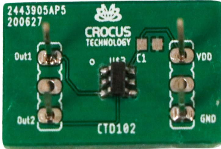
Figure 2: EVB102 SOT23-6 Evaluation Board
