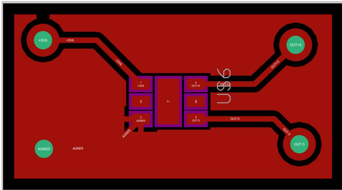
Figure 4: EVB102 SOT23-6 evaluation board top layer
