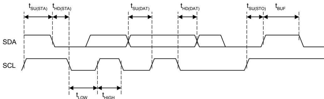
Figure 2: I<sup>2</sup>C input and output timing
