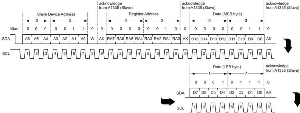
(2a) Load slave (A1335 device address 0x3) with EEPROM target data (0x123083) into EWD, then load register address 0x07:0x04)
