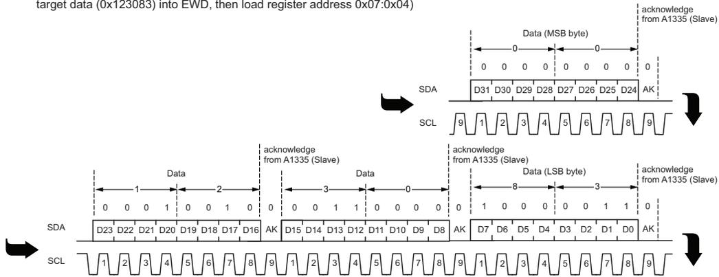
(3) Transfer (Write) slave (A1335 device address 0x3) EWD data into EEPROM (command: EXW (bit 15) set to 1 by sending 0x80 to EWCS register, address 0x08)
