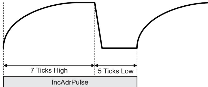
Figure 33: ASENT IncAdrPulse (Output by Host)
