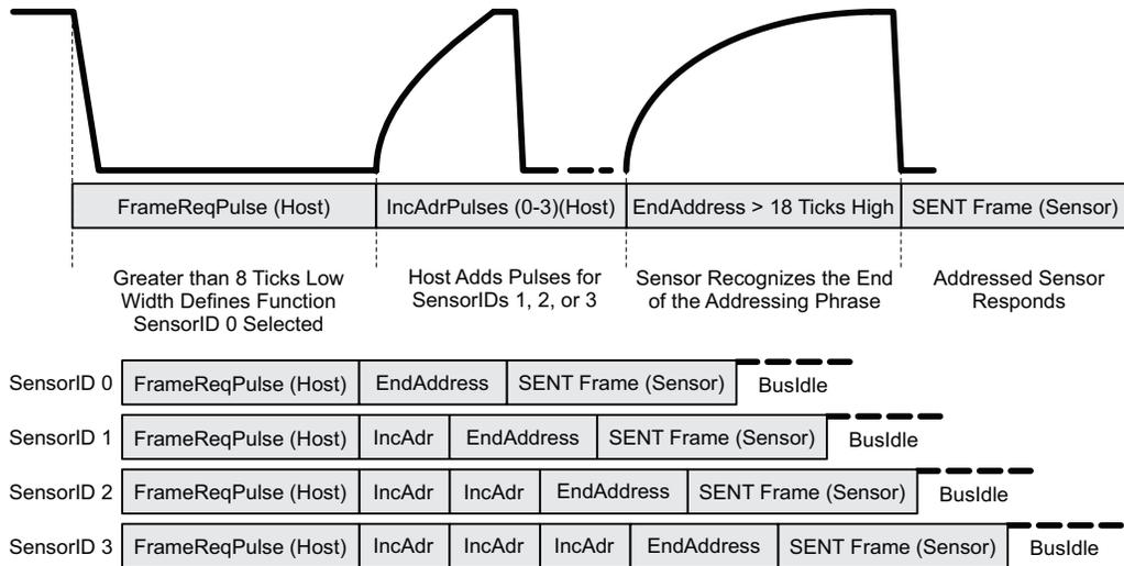
Figure 34: ASSENT Sensor Addressing
