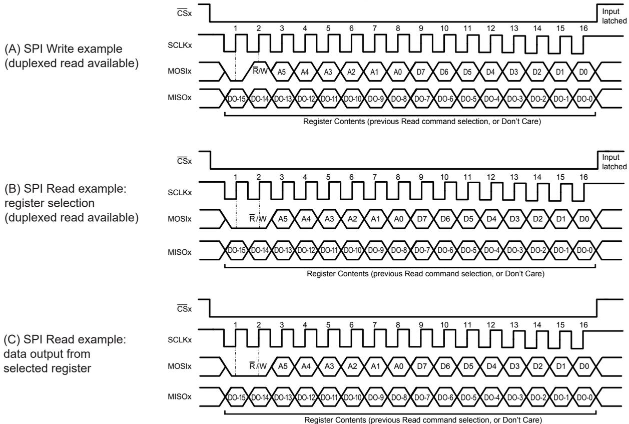
**Figure 9: SPI Read and Write Pulse Sequences**
