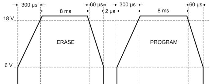
**Figure 17: V<sub>CC</sub> Pulse Profile for EEPROM Programming**
