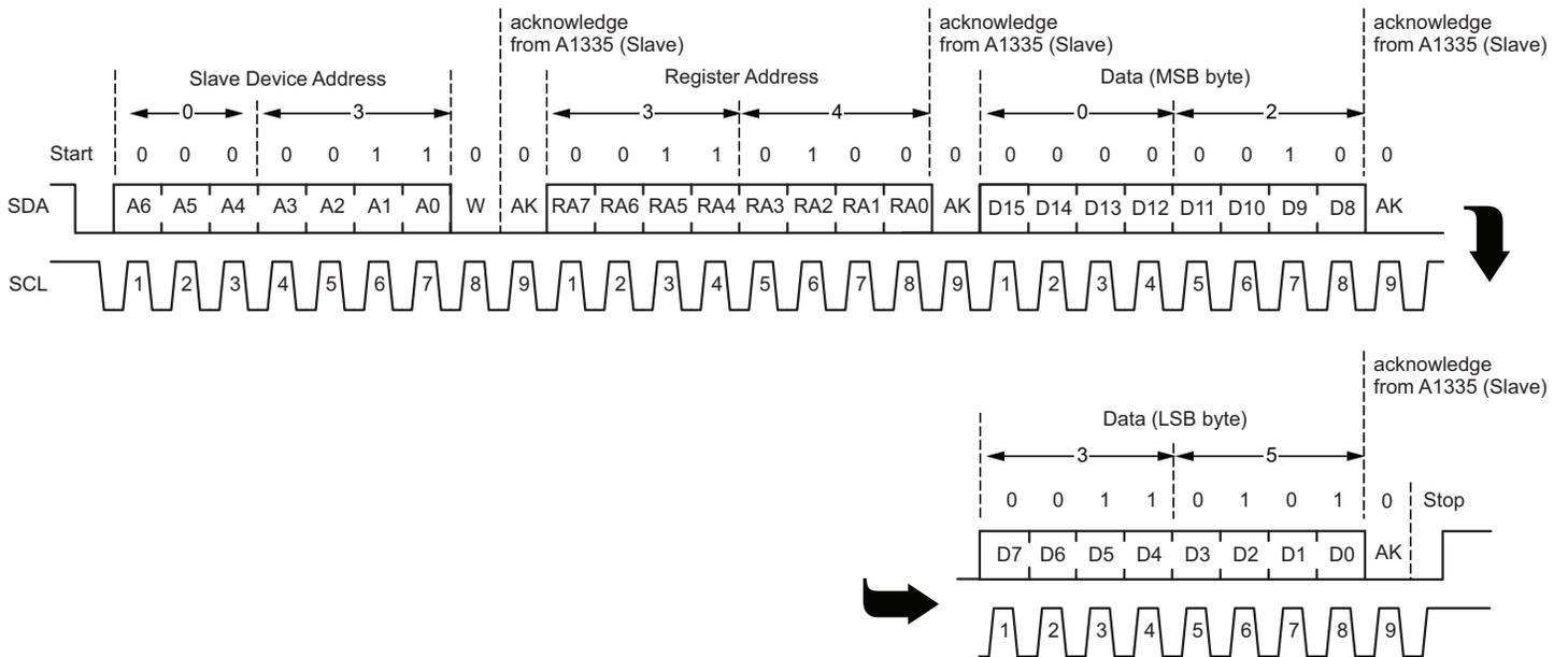
**Figure 4: I<sup>2</sup>C Base Address Write: value 0x0235 to register address 0x34 (ERM) in slave device 0x3.** All steps must occur immediately after the first step, with no intervening transmissions.
