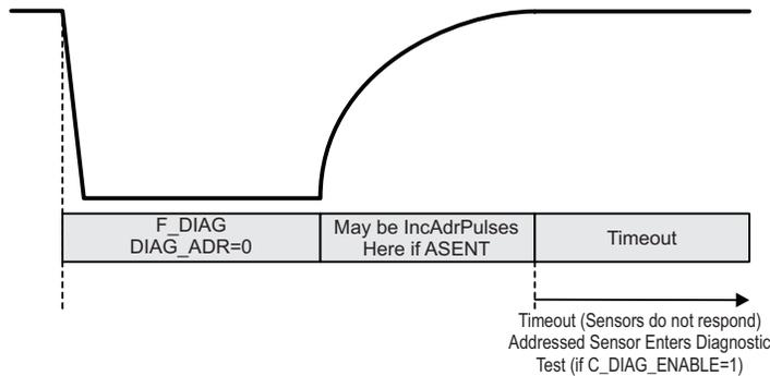
**Figure 39: Addressed Diagnostic Request for ASENT and SSENT**
