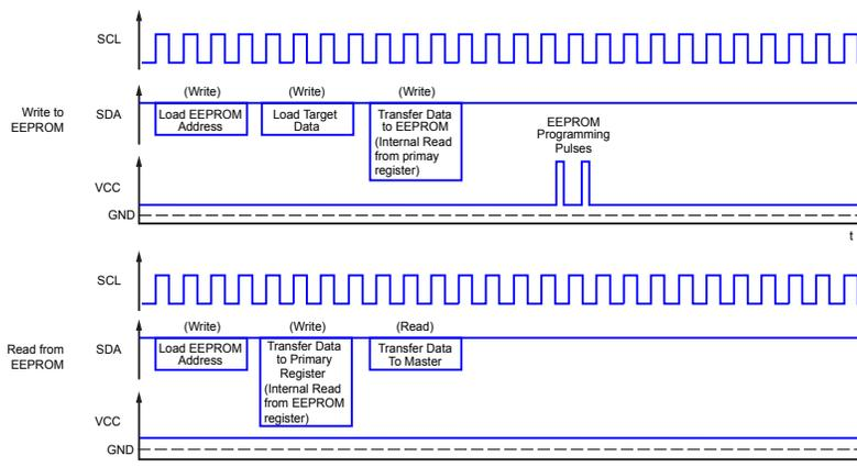
Figure 14: I<sup>2</sup>C Extended Address Write and Read Sessions Examples
