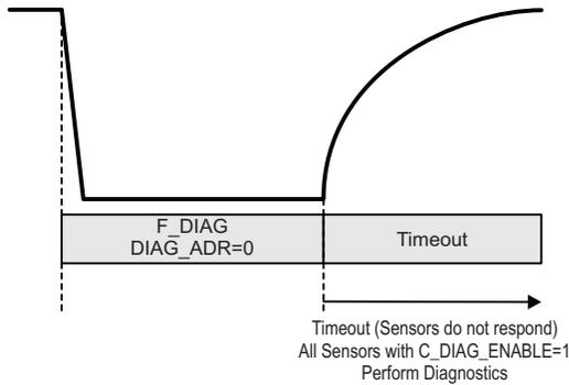
**Figure 38: Broadcast Diagnostic Request for ASENT and SSENT**
