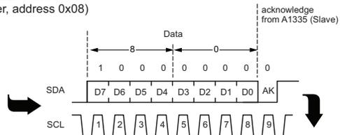
(4) Confirm Transfer (Write) slave (A1335 device address 0x3) EWD data into EEPROM (command: WDN (bit 0) Read the EWCS register, followed by dual programming pulses (not shown here))
