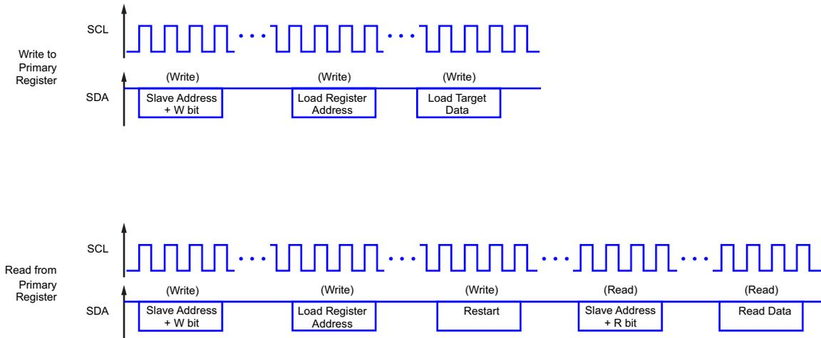
**Figure 3: I<sup>2</sup>C Base Address Write and Read Sessions Examples.**
