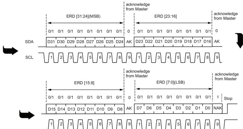
Figure 16: I<sup>2</sup>C Extended Address Read Example
