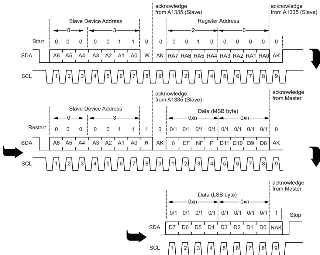
Figure 5: I<sup>2</sup>C Base Address Read: angle value and error status from register address 0x20 (ANG) in slave device 0x3. All steps must occur immediately after the first step, with no intervening transmissions.
