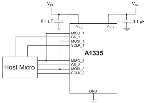
**Figure 41: Separate SCLK Lines**
