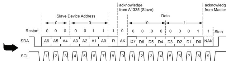
Figure 15: I<sup>2</sup>C Extended Address Write Example
