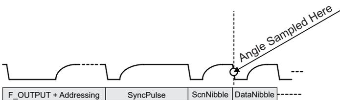
Figure 35: SampleOnOutput Example
