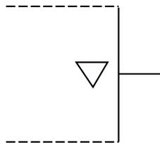
totem-pole output: A bipolar output whose active devices are so controlled that as the resistance of one increases, the resistance of the other decreases so that, according to the relative states of the two active devices, the output voltage can swing between levels approaching the two supply voltages.
