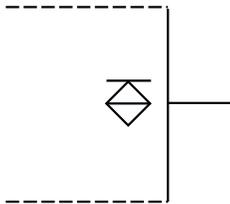
NOTE — The bar above the diamond indicates that the output is at the high logic level when the active device is in its on state.
