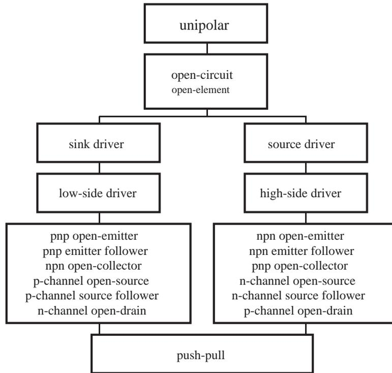
Figure 2 — Hierarchy of unipolar outputs
