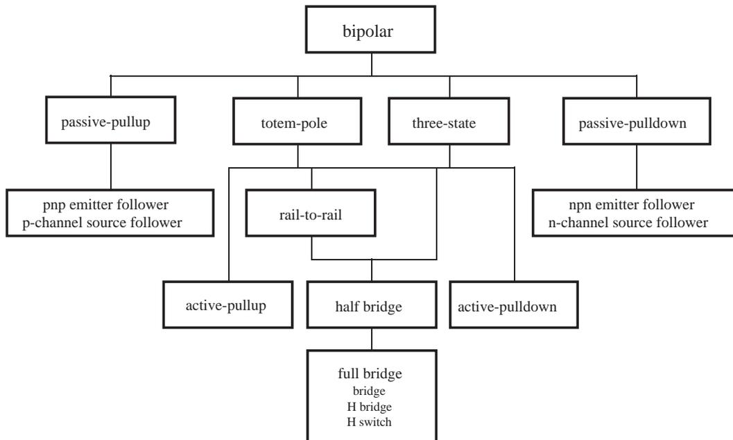
Figure 1 — Hierarchy of bipolar outputs
