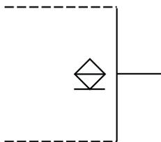
NOTE — The bar below the diamond indicates that the output is at the low logic level when the active device is in its on state.
