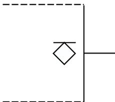
NOTE — The bar above the diamond indicates that the output is at the high logic level when the device is in its on state.
