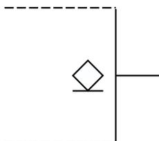
NOTE — The bar below the diamond indicates that the output is at the low logic level when the device is in its on state.
